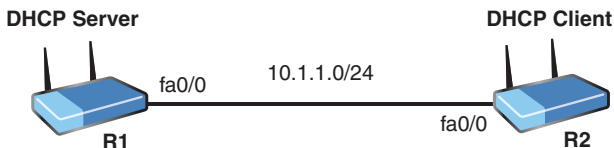
FIGURE 20.2 The DHCP Server and Client Topology
